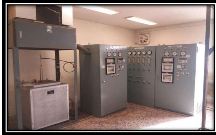
Fig. 4.1 A Reducibility testing system
