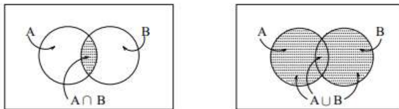
Figure 6: Venn diagrams for A \cap B (intersection), A \cup B (union).
